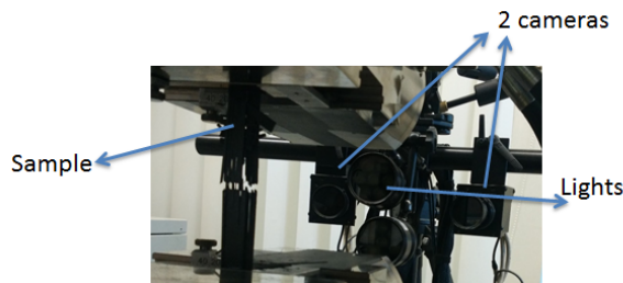
Figure 8.4. View of the sample and DIC equipment.
