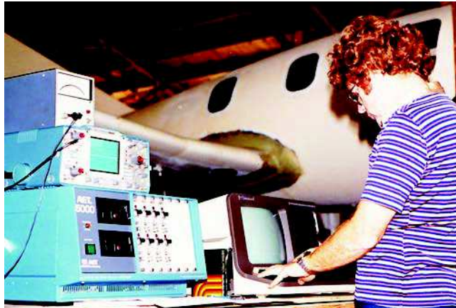
Figure 25 AE monitoring of prototype Avtek aircraft in 1984. Dr. I. Roman, on leave from Hebrew University of Jerusalem, operated AET-5000 system. [The original of the cover photo shown in JAE vol. 3]
