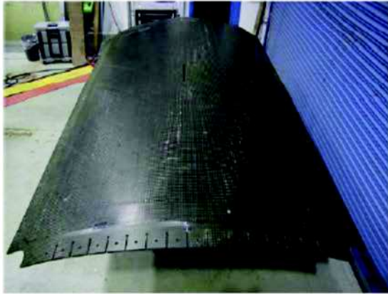
Fig. 27 Left: Honeycomb sandwich composite panel. Right: A segment of the panel showing the AE sensors arrangement, a photogrammetry system and an artificial notch. [177]
