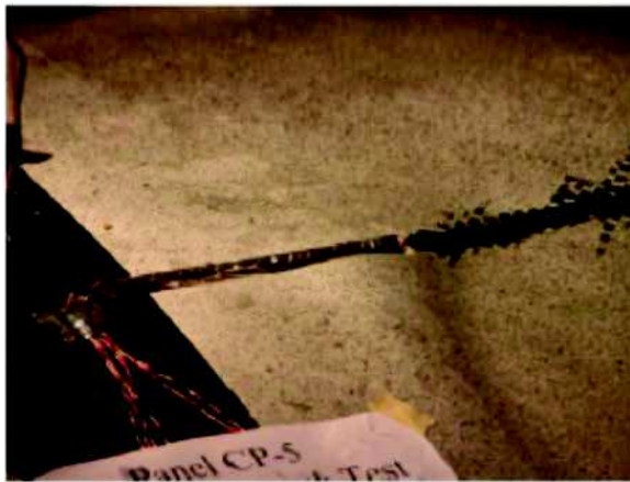
Fig. 28 Notch-tip damage after complete final fracture in two sandwich panels. [177]
